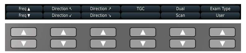
**Freq** Frequency up and down allows you to change the frequency setting (probespecific). Higher frequencies = higher resolution, lower frequencies are used for deeper penetration. The current frequency is indicated in the upper right portion of the screen (a number followed by MHz).
