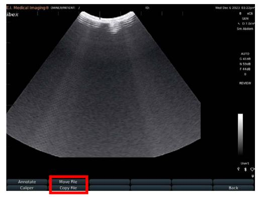
4 Press the corresponding **MOVE FILE** or **COPY FILE** button. Once completed, another dialog will display to show the operation completed.
