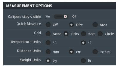
Calipers Stay Visible allows user to make a reference measurement on-screen that stays visible when the image is unfrozen
