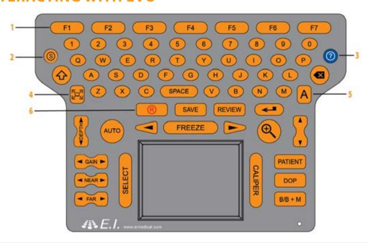
1 Function The FUNCTION keys [F1, F2 etc] coordinate with the on screen menu keys. For example, on the home screen, F1 is Exam Type.
