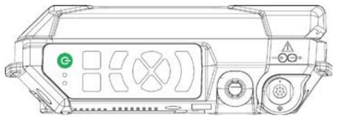
When used near an outlet, the EVO system can be powered directly [with or without the internal Li-lon battery pack installed] by the external power supply/battery charger. It may also be used outdoors [unsheltered locations] as an internally powered system with a charged internal Li-lon battery pack.
